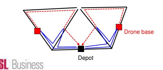
Each arc length = 2 Drone has capacity 5 Truck has capacity 6
